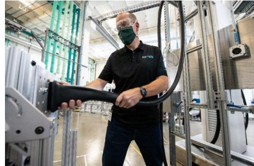
©NREL– Fit and ergonomics evaluation of the MCS
